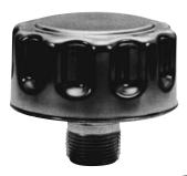
VESCOR® Screw-In Breathers insure free flow of air into hydraulic tanks or other fluid containers. These units let the tank breathe while keeping out airborne particles. Connection is ¾" NPT (male) for direct connection to standard ¾4" NPT (female) threaded pipe ports.
