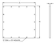
VESCOR<sup>®</sup> Multi Bolt Endcovers can be used on hydraulic reservoirs when a baffle is unavailable to mount a standard endcover and access to reservoir is required.
