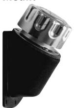
VESCOR® Side Mount Filler Breathers are designed to be used where top surfaces are not readily available for locating a filler port. This unit easily mounts on vertical tank walls. These units filter the fluid as it is added and also lets the tank breathe while keeping out airborne particles.
