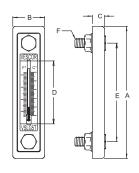
VESCOR VSLG5T (Economy) Series Sight Level Gauges are available in standard 5" size. Standard gauges are available with thermometer only and with standard front mount design.
