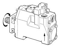
Fig. 4. Left hand rotating pump.
