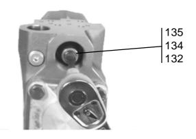
2. Remove the Hex S Screw (item 135), the Washer (item 134) and the Compression Spring (item 132). **Note!** The Bar is loctited with the Pivot Head and it might come loose when removeing the Hex S Screw (item 135).
