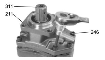
14. Install the Shaft (item 311), Bearing Housing (item 211), Swashplate (item 421) and Bar Assy (item 131). Hold the Swashplate against the Bearing Housing until the Splines on the Shaft enters the splines on the Cylinder Barrel. Assembly the Hex S Screws (item 246) according to the specified tightening torque 60±10Nm. "Note, to facilitate assembly use two longer screws and push the parts together until you can fit the original screws".
