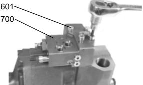
17. Install the LS Control (item 700). Tighten the screws (item 601) to the specified tightening torque  $24\pm5$ Nm.
