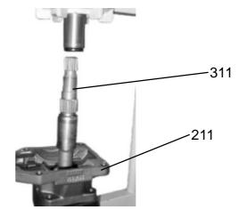
12. Place the Bearing Housing (item 211) on a tube (inside diameter 95 - 110mm) so that the Shaft (item 311) with Seal Carrier (item 231) can be pressed off. Press on the small shaft end. Remove the O-ring (item 225) from the Bearing Housing.
