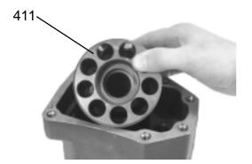
9. Remove the Cylinder Barrel (item 411).
