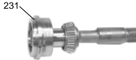
4. Install the Seal Carrier (item 231) on the shaft.
