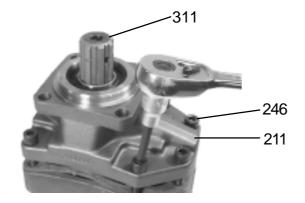
3. Remove the six Hex S Screws (item 246) and lift up the Shaft (item 311) with Bearing Housing (item 211).
