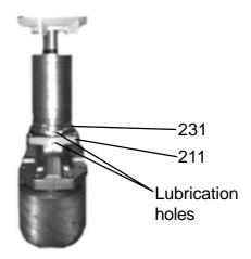
5. Install the O-ring (item 225) in the Bearing Housing (item 211). Install the Shaft with Seal Carrier in the Bearing Housing (item 211). Place the Bearing Housing on a tube (inside diameter 65mm and outside diameter max 80mm) and press down the Shaft with Seal Carrier. Press on the seal carrier and make sure that the lubrication holes are opposite eachother.
