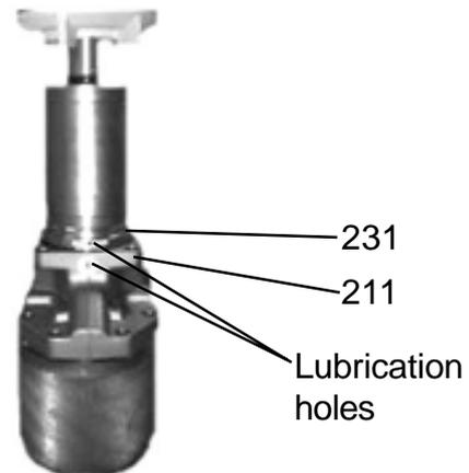
5. Install the O-ring (item 225) in the Bearing Housing (item 211). Install the Shaft with Seal Carrier in the Bearing Housing (item 211). Place the Bearing Housing on a tube (inside diameter 65mm and outside diameter max 80mm) and press down the Shaft with Seal Carrier. Press on the seal carrier and make sure that the lubrication holes are opposite each other.
