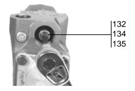
16. Install the Hex S Screw (item 135) together with the Washer (item 134) and the Compression Spring (item 132) according to the specified tightening torque 30±5Nm.
