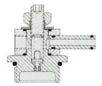
**Individual pressure limiters** limit the supply pressure to the section to a setting less than the system relief pressure, thereby protecting motors and cylinders.
