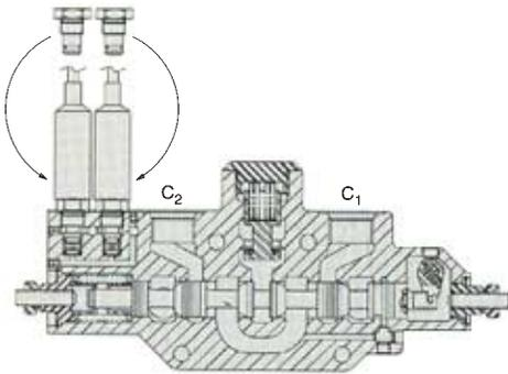
**Pilot oil operation** is achievable simply by installing optional fittings into standard bodies in place of the Pulsar solenoid cartridges.
