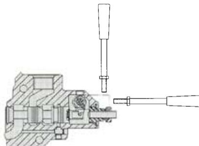
**Manual override is standard**, provides the user with a direct mechanical link to the main spool.
