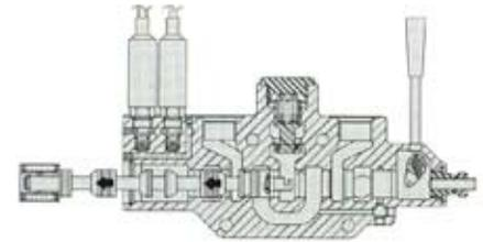
**Fully interchangeable spools\*** permit off-the-shelf changes of spools and flows from 2.5 to 40 gpm (9,5 to 151 L/min).
