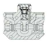
**Patented individual pressure compensation** is standard on all Pulsar VP/VPO Series sections — particularly useful when many functions will operate simultaneously.
