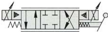
**Closed 4-way, 3-position spool** provides proportional control in each direction, typically for double-acting cylinders.
