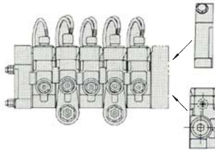
**Simply switch inlets** to change a stack from a load-sense to open-center application.
