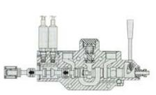
Fully interchangeable spools\* permit offthe-shelf changes of spools and flows from 2.5 to 40 gpm (9,5 to 151 L/min). \*VP spools cannot be used in VPO work segments and VPO spools cannot be used in VP work segments.
