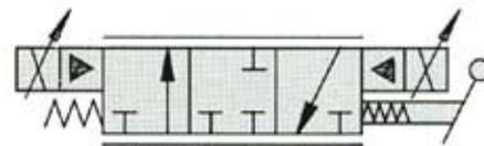
**Closed 3-way, 3-position spool** provides proportional, bi-directional control of single-acting cylinders. Spool is sized for flow force compensation at high pressure drops.
