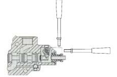
**Manual override is standard,** provides the user with a direct mechanical link to the main spool.
