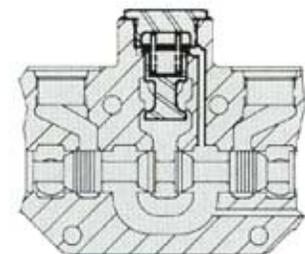
**Patented individual pressure compensation** is standard on all Pulsar VP/VPO Series sections — particularly useful when many functions will operate simultaneously.
