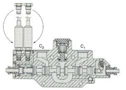
**Pilot oil operation** is achievable simply by installing optional fittings into standard bodies in place of the Pulsar solenoid cartridges.
