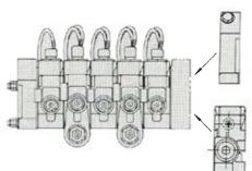
Simply switch inlets to change a stack from a load-sense to open-center application.
