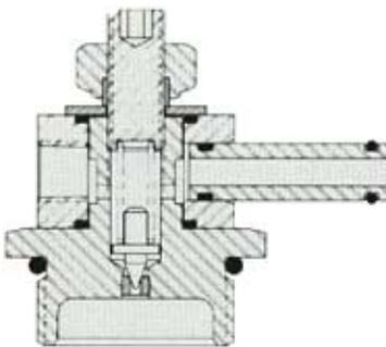
**Individual pressure limiters** limit the supply pressure to the section to a setting less than the system relief pressure, thereby protecting motors and cylinders.
