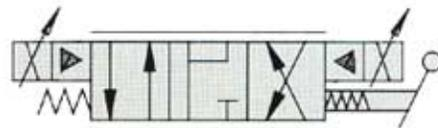
**Open (motor) 4-way, 3-position spool** provides proportional, bi-directional flow control. Permits free actuator movement in neutral.
