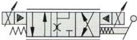
**Restricted open 4-way, 3-position spool** provides proportional, bi-directional flow control. Permits free actuator movement in neutral, but restricts flow to 1 gpm (3,8 L/min) at a 100 psi (7,0 bar) drop.
