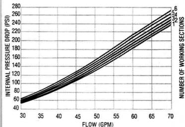
NOTE: VA models are constructed of grey iron and are rated for 2500 psi in 40 gpm (VA20) and 70 gpm (VA35) sizes. VG models are constructed of compacted graphite and are rated for 3500 psi service in corresponding gallonage sizes.
