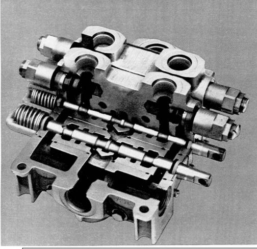
VA and VG model valves are contemporary versions of our well-proven A20/A35 units which have provided reliable control of fluid power for over 20 years. The VG models are cast from compacted graphite, a high strength iron alloy that allows us to rate the valves to 3500 psi. VA models are cast from gray iron and are rated at 2500 psi.
