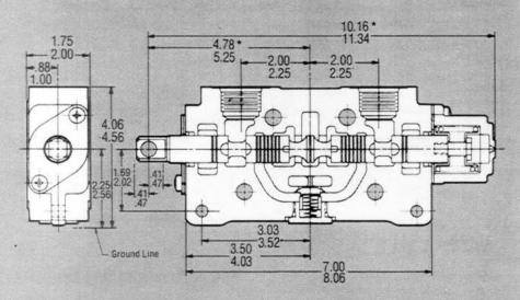
\* These dimensions are shown for a manually operated valve with spring return. See operators pages 12 and 13 for other combinations.
