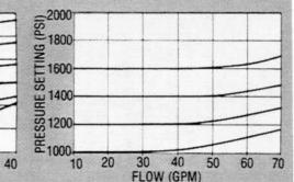
NOTE: Unless otherwise specified main relief valves will be screw adjusted.
