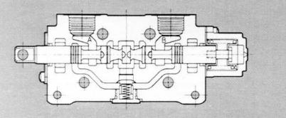
Commercial's VA and VG models are opencenter, stack type valves designed primarily for heavy-duty mobile equipment applications. They work equally well with fixed or variable displacement pumps.
