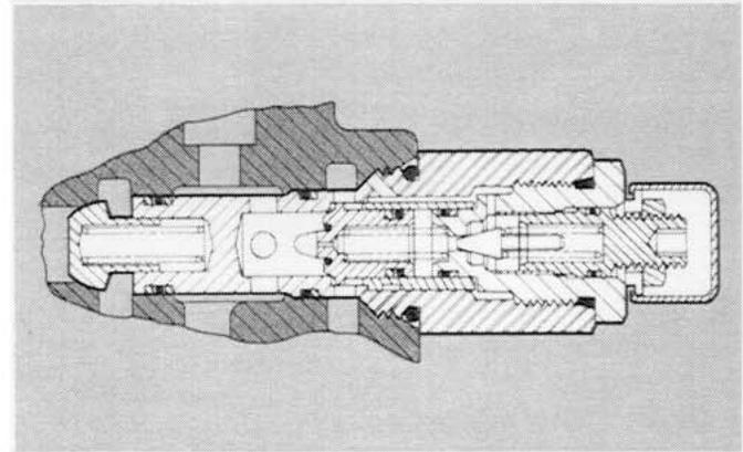
Model RP20 work port relief valves are pilot-operated type.
