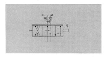
This work section and check valve are combined to perform the functions of a 4-way work section and a pilot-operated check or lockout valve in one single housing.
