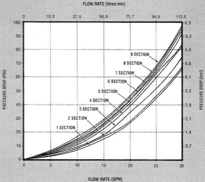
Curves derived from actual laboratory tests run with 150 SUS oil, at 100°F [38°C].
