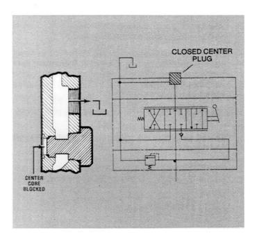
same, only one relief valve is required. It must be installed in the upstream valve.
