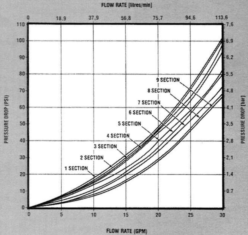
Curves derived from actual laboratory tests run with 150 SUS oil, at 100°F [38°C].
