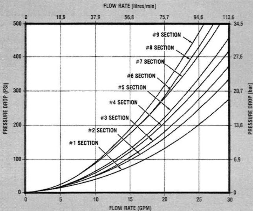
Curves derived from actual laboratory tests run with 150 SUS oil, at 100°F [38°C].
