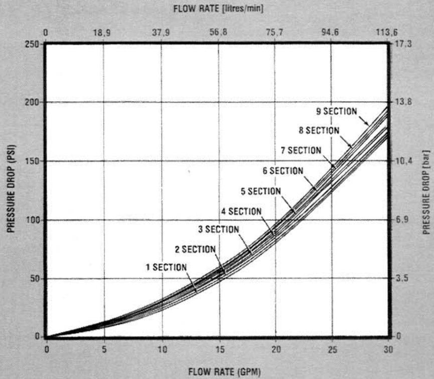
Curves derived from actual laboratory tests run with 150 SUS oil, at 100°F [38°C].
