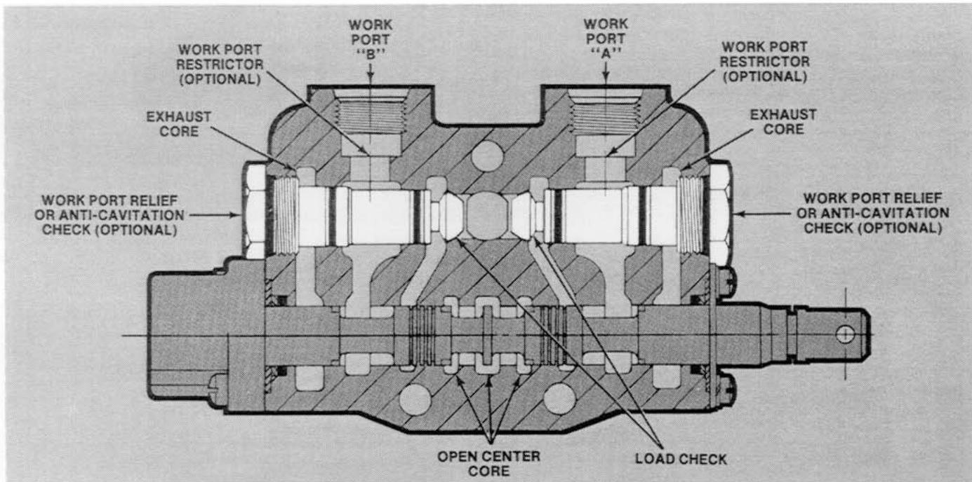
In addition to load checks which are standard in the V20 Valves, Gresen offers a wide range of options to control oil flow. From these options you may select the exact accessories to customize your valves to your specific application.
