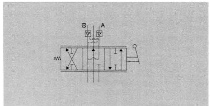
This work section and check valve are combined to perform the functions of a 4-way work section and a pilot-operated check or lockout valve in one single housing.
