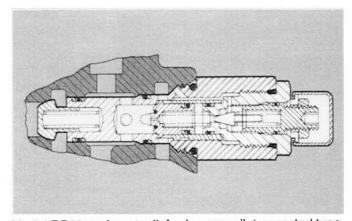
Model RP20 work port relief valves are pilot-operated type.
