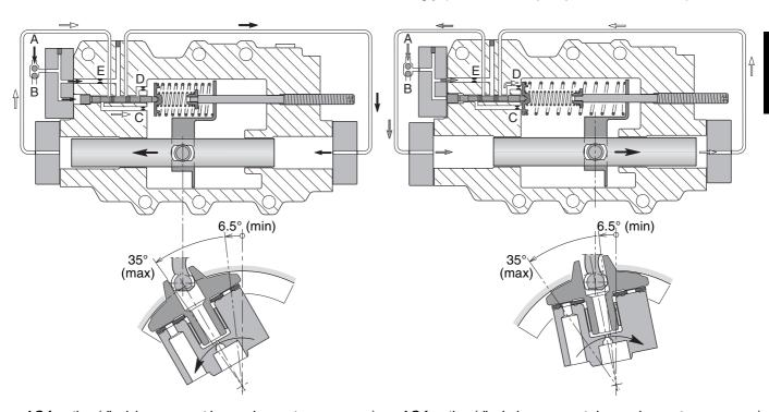
AC function (displ. increases at increasing system pressure).
