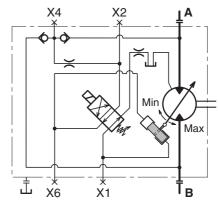
EO H 01 I schematic (non-activated solenoid).
