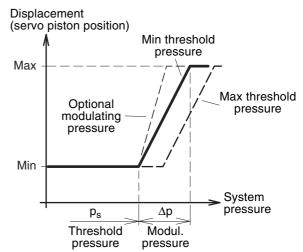
AC diagram (displacement vs. system pressure).
