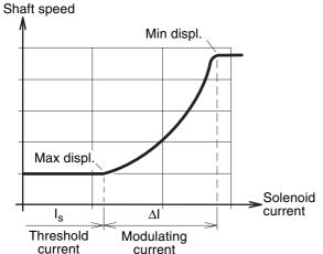
Please note: The shaft speed is **not** proportional to the solenoid current.
