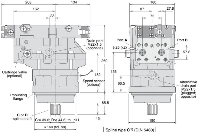
\* Measurement valid for spline type C. Corresponding measurement for spline type D is 5 mm longer.
