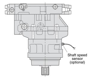
V14-110 (AC control) with speed sensor.
