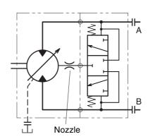
T12 with flushing valve block type FV.
