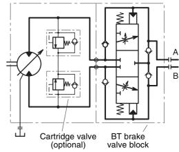
T12 with cartridge valves and brake valve block type BT.
