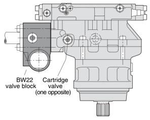
V14- 110 (AC control) with BW22 valve block.
