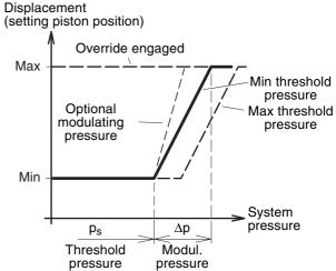
AH diagram (displacement vs. system pressure).
