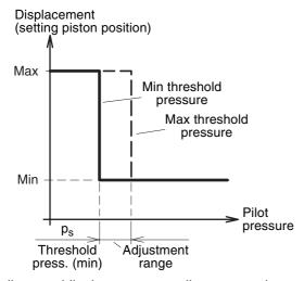
HO diagram (displacement vs. pilot pressure).
