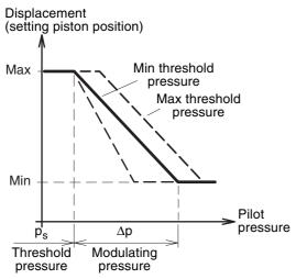
HP diagram (displacement vs. pilot pressure).
