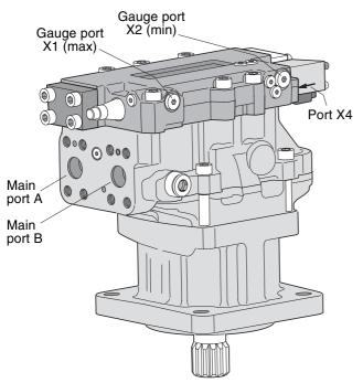
Gauge ports (EO and EP controls):
