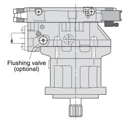
V14-110 (EP control) with built-in flushing valve.
