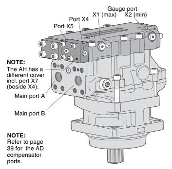
Gauge/pilot ports (AC and AH compensators):
