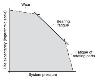
Hydraulic motor life versus system pressure.
