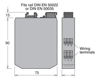
Electronic module (incl. internal programming module).
