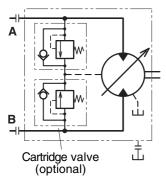
Hydraulic schematic - V14 with cartridge valves.
