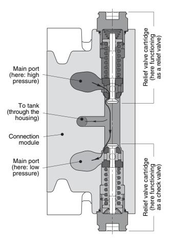
Section A-A (showing pressure relief cartridges).
