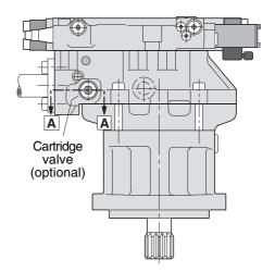
V14- 110 (EP control) with relief valve cartridges.
