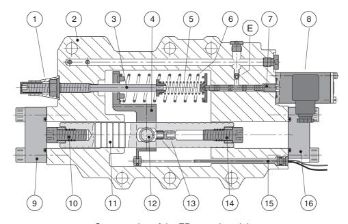
Cross section of the EP control module.
