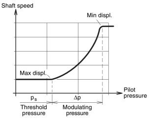
Shaft speed vs. pilot pressure (HP control).
