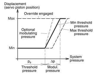
AH diagram (displacement vs. system pressure).
