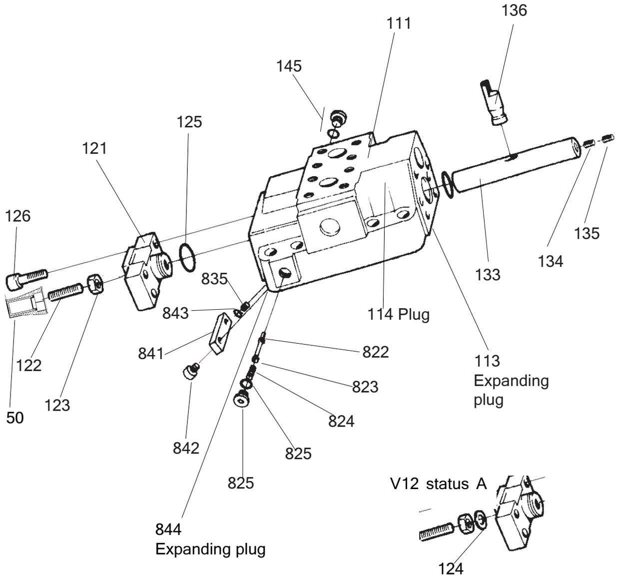
V12 status B, *companion pin, item 136 is located by a detent ball and a spring and displacement limiters are installed in the ends of the Setting Piston.*
