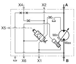
HO S 01 E schematic (X5 not pressurized).
