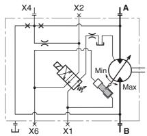
EO H 01 E schematic (non-activated solenoid).
