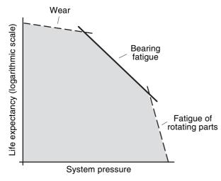
Hydraulic motor life versus system pressure.
