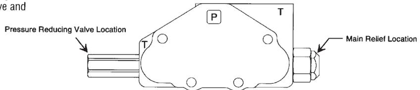
No. 23613 Inlet Cover for all Solenoid-Operated Valves
