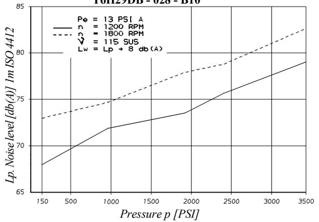
Noise level is given with each cartridge discharging at the pressure noted on the curve (P1 full flow).
