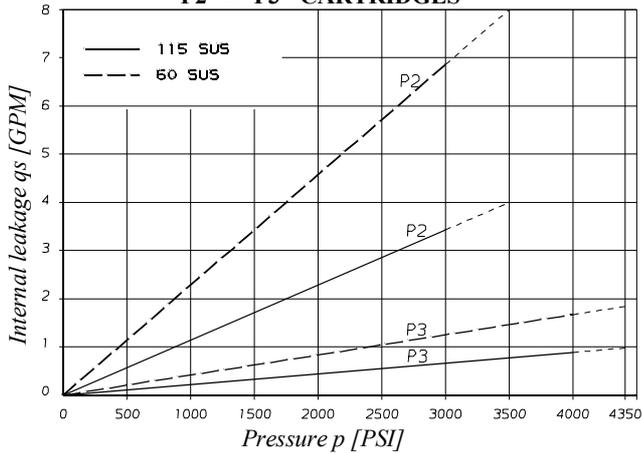
Do not operate pump more than 5 seconds at any speed or viscosity if internal leakage is higher than 50% of theoretical flow.
