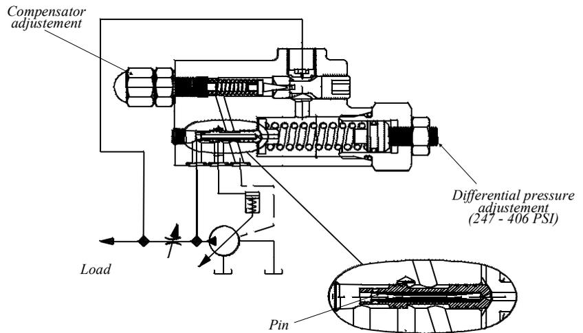
**X - VENTED COMPENSATOR BY ELECTRIC VALVE**
