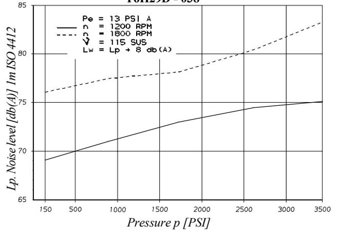
Noise level is given with each cartridge discharging at the pressure noted on the curve (P1 full flow).
