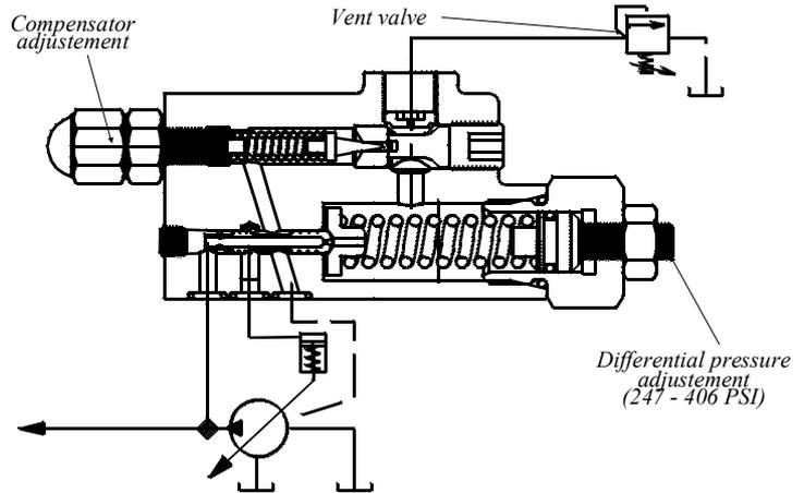
**L - LOAD SENSING COMPENSATOR**
