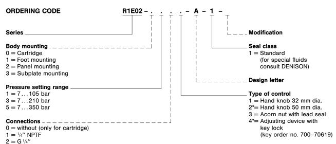
$^{\star}$  = on bodies for subplate mounting use adapter plate S16-64188 if necessary. The following 4 valve mounting srews are necessary then: M10 x 55
