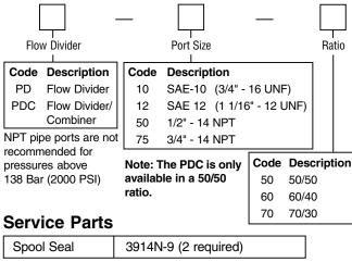
Note: The body and the internal parts are non-service items. PD-PDC.p65, dd
