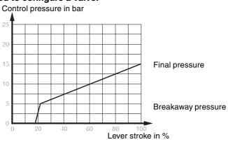
*Diagram shows an example of a straight characteristic.* Control pressure in bar
