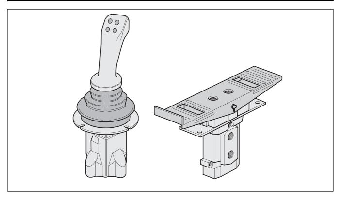
The PCL4 is a stackable hydraulic control-pressure valve intended for the proportional, hydraulic remote control of directional valves, pumps with variable displacement, positioning cylinders, etc. It can be obtained with a co-ordinate lever (joystick), linear lever or foot pedal as the activating device.
