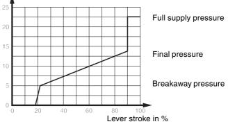
Diagram shows an example of a straight characteristic with overtravel stroke that gives full supply pressure. Control pressure in bar
