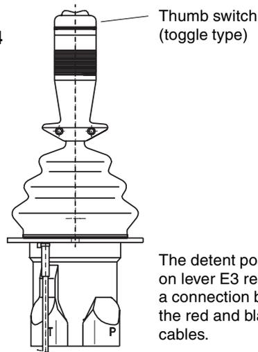
The detent position on lever E3 results in a connection between the red and black cables.
