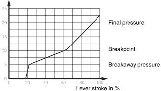
*Diagram shows an example of a broken characteristic.* Control pressure in bar
