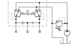
Signal obtained in port S on activation of valve.
