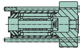
This spool positioner uses hydraulic pressure against the area of the spool, opposed by a spring, to achieve metering control. The design permits the constant transfer of oil from the cap to the tank core of the work section to help warm the oil during cold weather start-up. For optimum performance, it should be matched with a controller that has a spring pack of 95-400 psi (7-28 bar). Stroke limiters are available when the pilot ports are machined perpendicular to the spool.
