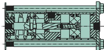
This spool positioner uses air pressure plumbed to a double-acting piston on one end of the spool to shift the spool in both directions. The other end of the spool is available for alternate actuation methods. The pressure range is 100 psi min. (7 bar) and 150 psi max (10 bar). The approximate metering range is 15-75 psi (1-5 bar).
