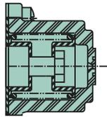
A spring in the end cap of this standard spool operator returns the spool to neutral from either work position when the control handle is released.
