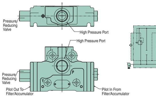
External pilot for the option of plumbing thru a filter (supplied by customer) and then back into the inlet. Pilot pressure is then internal to the A and B sides of the valve.
