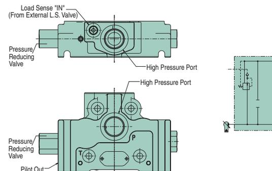
External pilot only with a check for operation with an accumulator (supplied by customer).
