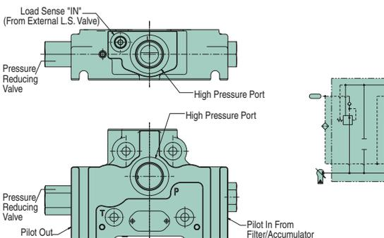
Same as Code R2, except has a check for operation with an accumulator (supplied by customer). When pressure falls below a defined level, the check closes and the accumulator supplies pilot pressure to the valve.
