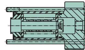
This spool positioner uses hydraulic pressure against the area of the spool opposed by a spring. The design permits the constant transfer of oil from the cap to the tank core of the work section to help warm the oil during cold weather start-up. Recommended pilot pressure input is 300-500 psi (21-34 bar) above tank pressure.
