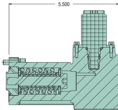
This spool positioner has a cap and solenoid on each end of the spool. The pilot and drain can be internal or external. This picture shows internal pilot and drain. The caps are also available with stroke limiters. The solenoids are available in 12V and 24V with the option of manual operation via a push-pin. The solenoid connector is AMP Junior. The same solenoid is used for on/off or proportional operation.
