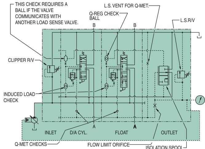
The relief valve in the inlet is referred to as a clipper relief. Its purpose is to clip the spikes normally associated with the de-stroking of piston pumps. When the clipper relief valve opens, all of the pump flow is returned to tank. It should always be set at least 500 psi higher than the load-sense relief-valve to ensure optimum performance.
