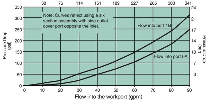
**Meter - In Flow to Workport Manual Operated Worksections**
