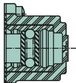
This option allows the spool to be detented in neutral and both of the power positions. Spool movement from one position to another is done manually.
