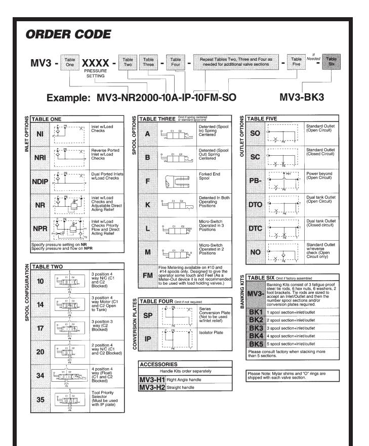
HOW TO ORDER: Parker Mini-Pak Valves are coded by the assembled stack configuration (Left to Right) in a sequential order from inlet to outlet. Please refer to the ordering tables, to select a circuit type, inlet options, spool configuration, spool options, circuit conversion options as they apply to your application.
