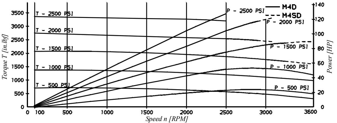
**DIMENSIONS & OPERATING CHARACTERISTICS - Weight : 59.5 lbs - M4D - M4SD SERIES**
