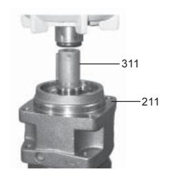
Place the bearing housing (item 211) on a tube
