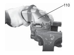
Lift off the barrel housing (item 110). Make sure that the valve plate doesn't fall out when lifting the barrel housing off.
