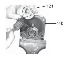
Put some grease on the valve plate (item 121) and install it into the barrel housing (item 110).
