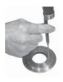
Tap the shaft seal out with hammer and mandrel.
