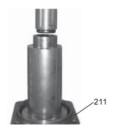
Push on the bearing ring (item 460) in the bearing housing (item 211) with a press. Use a tube to match the outer diameter off the bearing ring.
