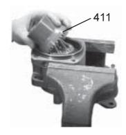
Install the cylinder barrel (item 411). Ensure correct timing. (Marking, punch mark)
