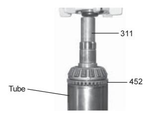
Place the ring gear (item 452) on a tube. Push out the shaft (item 311) with a press.
