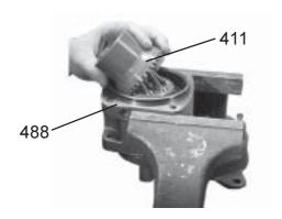
Lift off the cylinder barrel (item 411). Take the shim (item 488) away.
