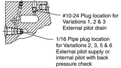
**Note:** 41.9mm (1.65") from bottom of bolt counterbore.
