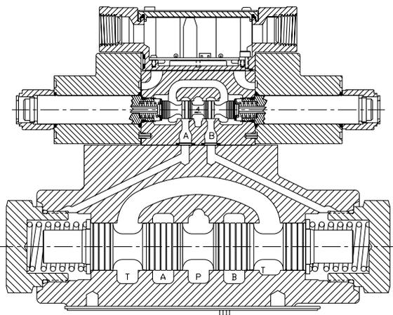
**D61\*W Solenoid Operated Conduit Box Style**
