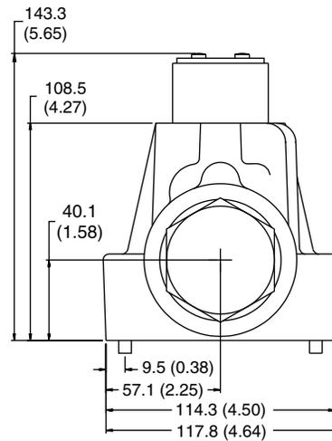
**Pilot Operated with Pilot Choke Control**
