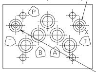
1/16 Pipe Plug for Variations 4 & 5 Torque to:  $11.67 \pm 1.67$  Nm ( $105 \pm 15$  in-lbs)
