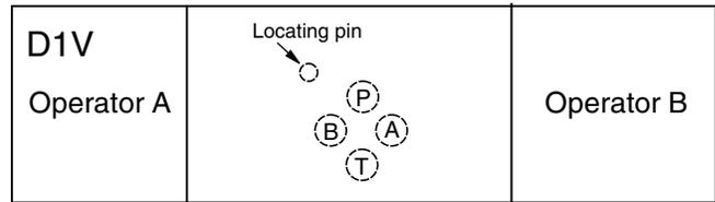
\*Note: On valves with 008 or 009 spool, A and/or B operators reverse sides. Flow paths remain the same as viewed from top of valve.
