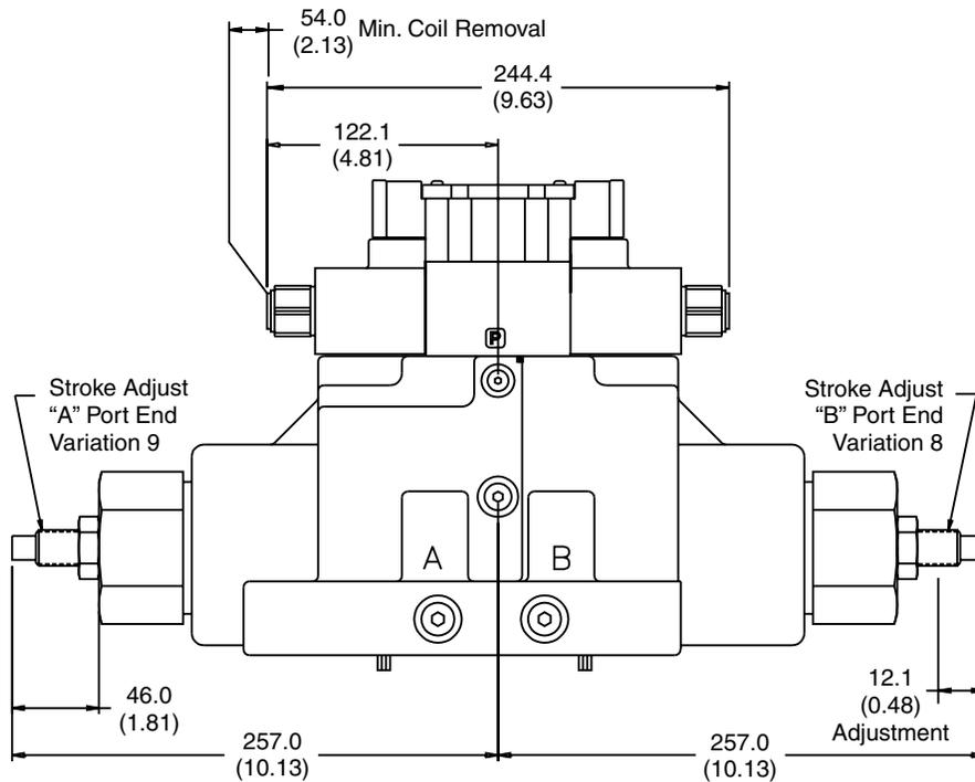
**Hirschmann and Pilot Choke Control, Double DC Solenoid**
