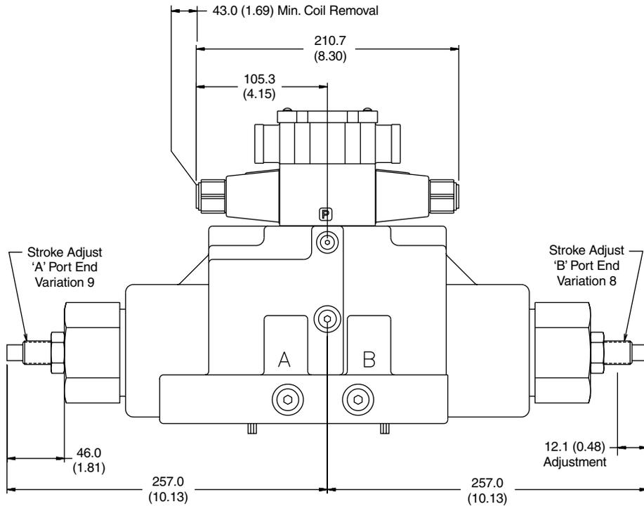
Conduit Box and Pilot Choke Control, Double AC Solenoid
