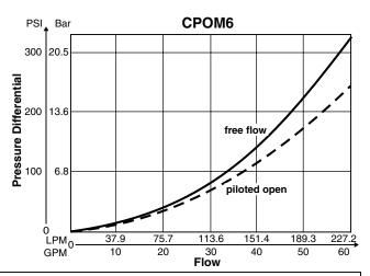
Curves were generated using 100 SSU hydraulic oil. For any other viscosity, pressure drop will change as per chart.
