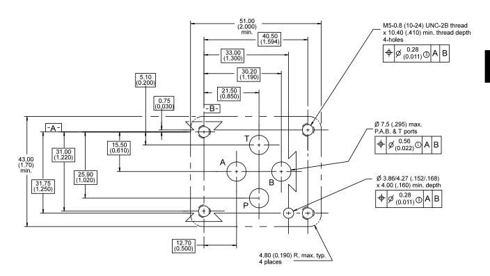
Mounting Surface for Directional Control Valve Manifold M'TD. (NFPA, D03); CETOP 3 & NG 6
