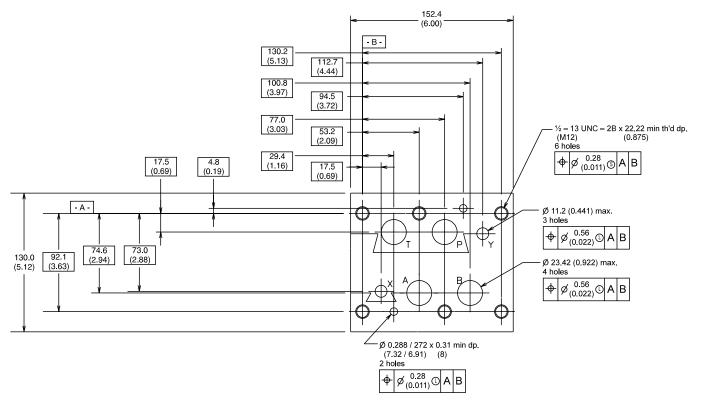
Mounting Surface for Directional Control Valve (NFPA, D08); CETOP 8 & NG 25
