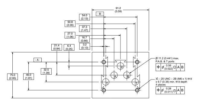
Mounting Surface for Directional Control Valve (NFPA, D05); CETOP 5 & NG 10
