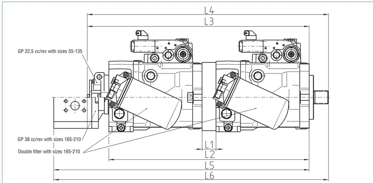
In case of tandem pump configuration the required size of the boost pump depends on the actual application. Criteria e.g. are diesel engine speed, number of hydraulic motors fed, working cycles.
