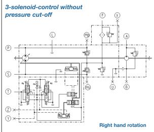
P, S High pressure portsA Pressure port, boost pumpB Suction port, boost pump
