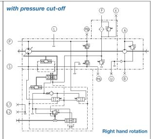
**P,S** High pressure ports **A** Pressure port, boost pump
