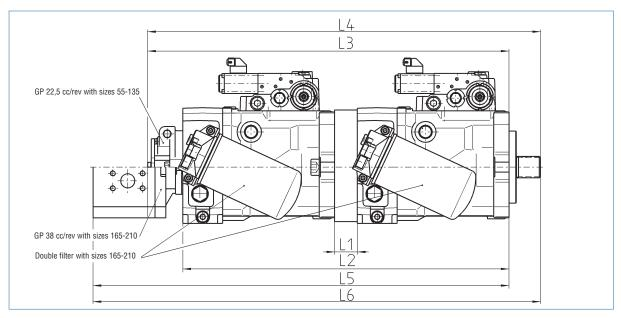
In case of tandem pump configuration the required size of the boost pump depends on the actual application. Criteria e.g. are diesel engine speed, number of hydraulic motors fed, working cycles.
