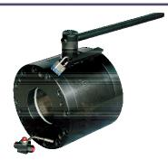
DMIC's Fixed Flange Ball Valves in SAE, DM-Flange, ANSI, and DIN patterns solve the problem of derated SAE working pressures in large sizes. Standard production is up to 6" size, with special order valves available to 12 inch or more, with up to 6000 PSI working pressure.
