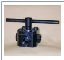
DMIC 'BV3H' and 'BV4H' series have been upgraded for superior performance and durability with DMIC's exclusive top servicable design, SpindleStack III™ needle bearing construction, and compatibility with many DMIC Pre-Engineered Accessories and Actuation Packages. This model is not restricted to any specific type of circuit, and incorporates BLOCKED CENTER (intermediate) positions.
