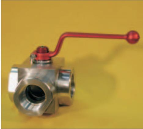
The 'BV3L' is an economical U.S. made diverter valve for Filter Duplexing type applications where one input is directed to one of two outputs. Standard "L-Bore" ball with slight port overlap prevents upstream pressure spikes during phase change.
