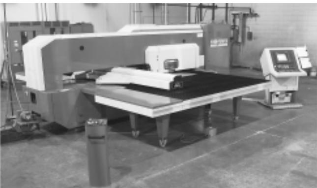
*One of three CNC sheet metal fabrication cells for standard and custom products.*
