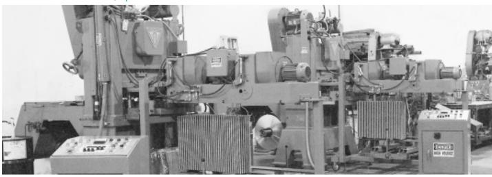
View of several high capacity air-cooler fin making machines. Provides high technology fin pattern with variable spacing capability.
